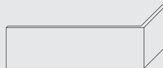
StoCleyer B corner resin brick slip normal format: 240/115x71 mm
